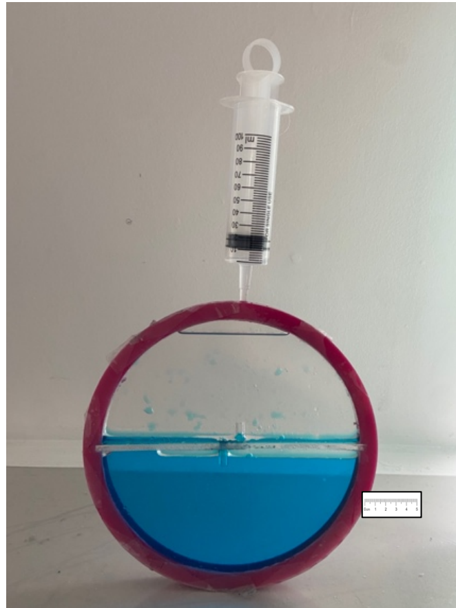
Figure 25 - filling up refined prototype (3% glycerol composition) with syringe
