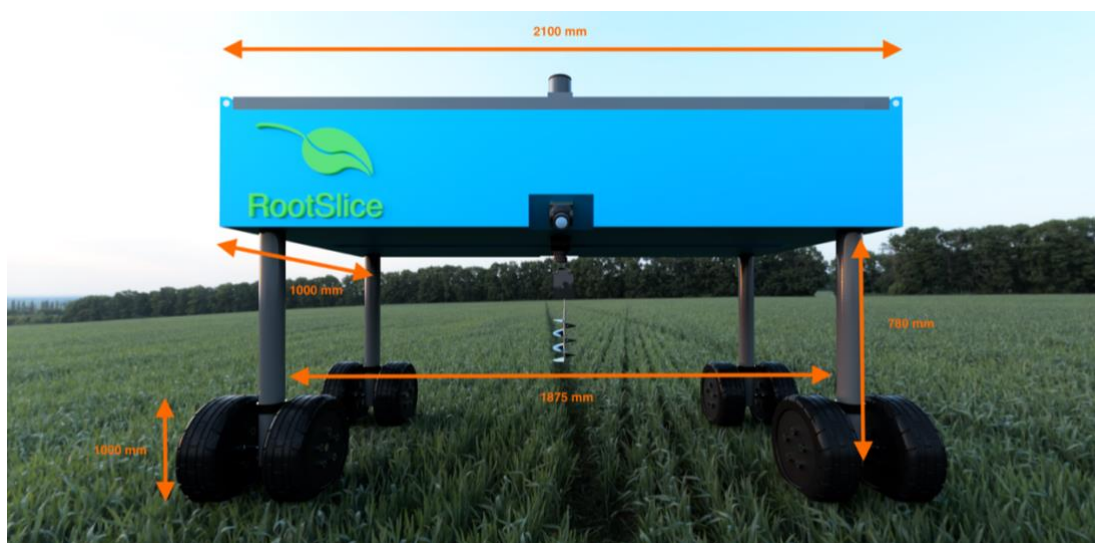
Figure 5 – Robot model without accessories, showing the overall dimensions
