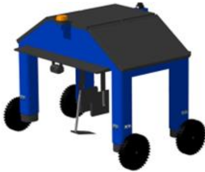
Figure 3 – Initial CAD of the rover with the 'dig and grab' mechanism (open position).
