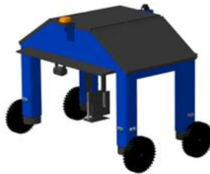
Figure 4 – Initial CAD of the rover with the 'dig and grab' mechanism (close position)
